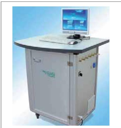
**The CamScan Mobile** is a mobile analysis unit for the automatic testing of an installed filter. As defined in the standard DIN 1822, the built-in filter can be tested for overall separation efficiency and any possible leaks. The computer that is integrated into the system stores the measurement values, which in turn allows for trouble-free documentation.
