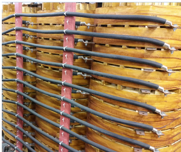
Figure 5: Typical Frame 4 (4000-6000HP) Input Transformer
