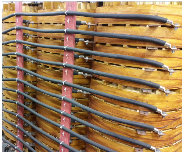
Figure 5: Typical Frame 4 (4000-6000HP) Input Transformer
