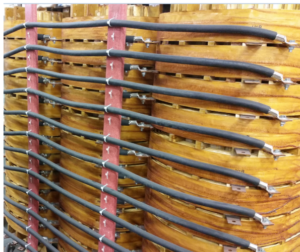
Figure 5: Typical Frame 4 (4000-6000HP) Input Transformer
