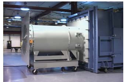
PHOTO C. Variable-supply and exhaust system used in an ANSI/AMCA Standard 210-99 test.
