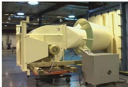
PHOTO A. High-plume dilution blower mounted on the inlet of a test chamber in an AMCA-accredited laboratory.
