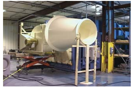
PHOTO B. High-plume dilution blower mounted on the outlet of a test chamber in an AMCA-accredited laboratory.
